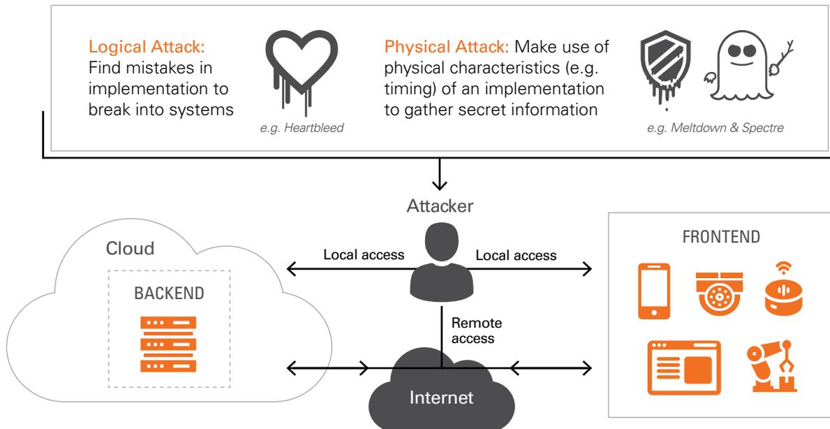
When hackers try to break a system, they carry out implementation attacks on hardware or software, thereby using logical or physical attack principles applied locally or remotely.
